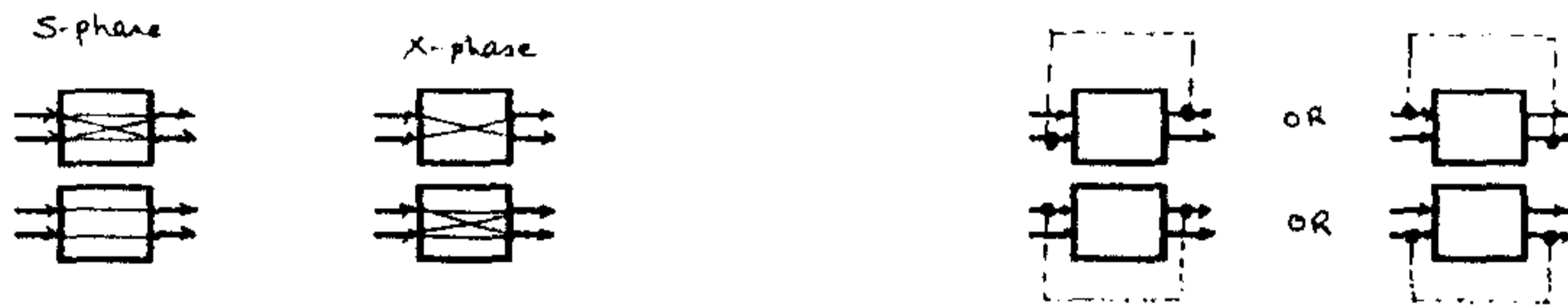
Fig. 16. Non separated two-response fault : undistinguishable SE and two-link short circuit fault. (a) Fault observed in S-phase. (b) Fault observed in X-phase.
