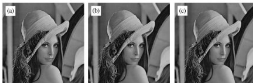
Fig. 3. Output images after pattern fitting: (a) A, d (PSNR= 31.79, bpp= 1.375) (b) A, d' (PSNR= 31.61, bpp= 0.88) (c) A', d' (PSNR= 31.57, bpp= 0.64).
