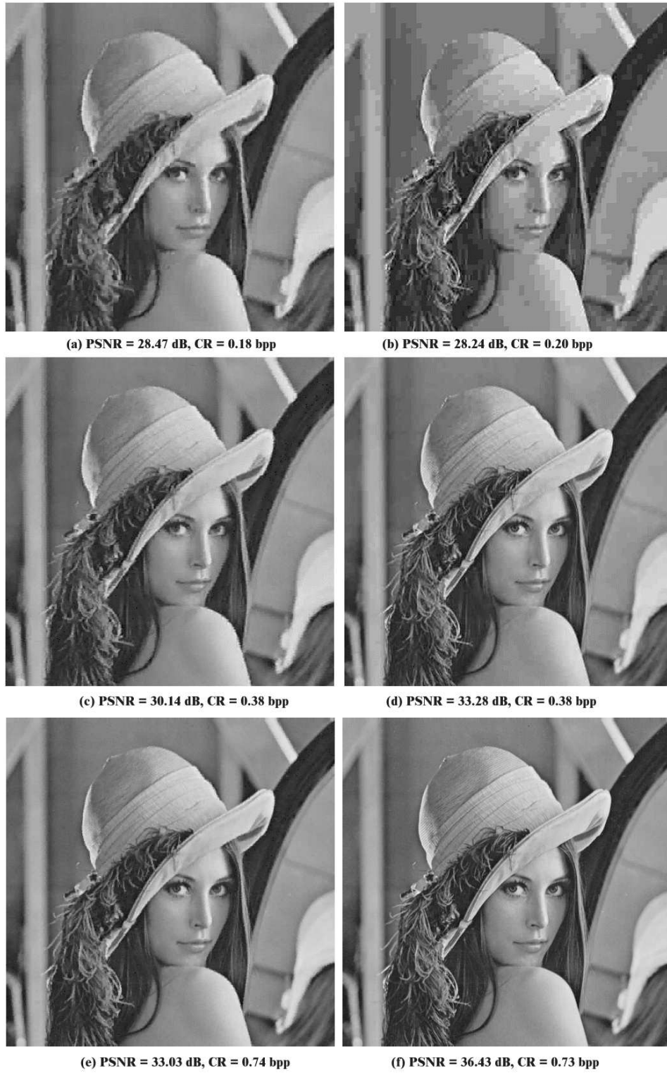
Figure 7.8: (a), (c), (e) Compressed Lena images using proposed algorithm. (b), (d), (f) Compressed Lena images using JPEG.
