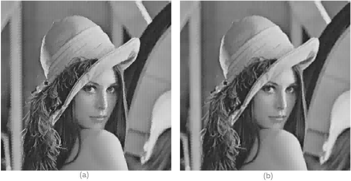
Figure 7.4: (a) Reconstructed Lena image with VQ using SOM weight vectors as reconstruction vectors. PSNR = 28.19 dB. (b) Reconstructed Lena image with VQ using surface fitting. PSNR = 28.49 dB.
