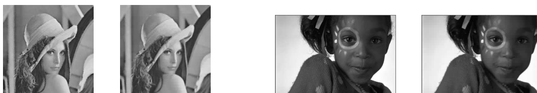
Figure 13. Original and decompressed image of (i) lena with compression 96.43% and PSNR 32.81; (ii) girl with compression 95.66% and PSNR 34.27
