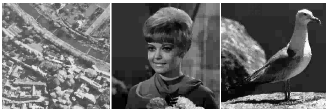
Figure 7. (Left to right): (i) decoded LFA, 1.79 bpp, where subimage size is 2 \times 2 , (ii) decoded Girl, 0.76 bpp, where subimage size is 2 \times 2 , and (iii) decoded Seagull, 1.11 bpp, where subimage size is 2 \times 2
