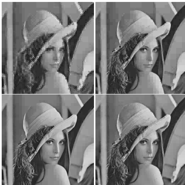
Figure 6. Decoded Lena (clockwise from top left corner): (i) 0.40 bpp, where subimage size is 4 \times 4 ; (ii) 0.90 bpp, subimage size is 2 \times 2 ; (iii) 1.58 bpp, where subimage size is 2 \times 2 ; (iv) 2.50 bpp, where subimage size is 2 \times 2
