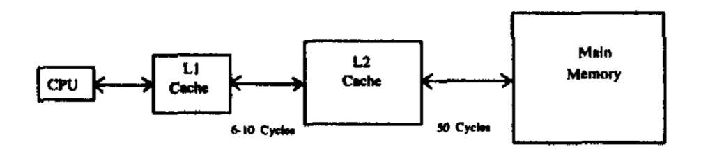
Figure 1: A Computer With Two Levels of Cache
