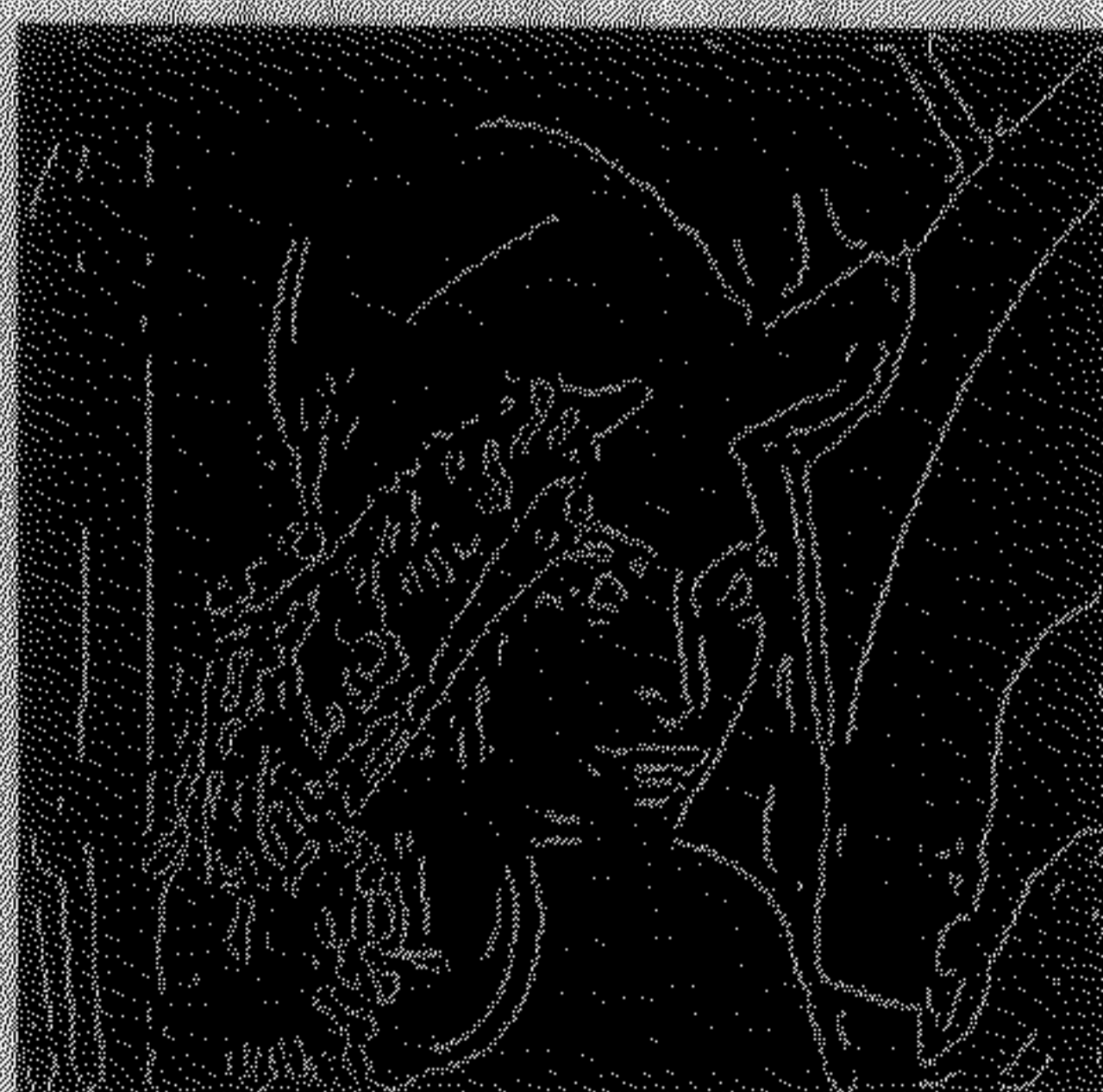
Figure 3.4: Edge detection by neural learning when target was edge image by Canny operator.
