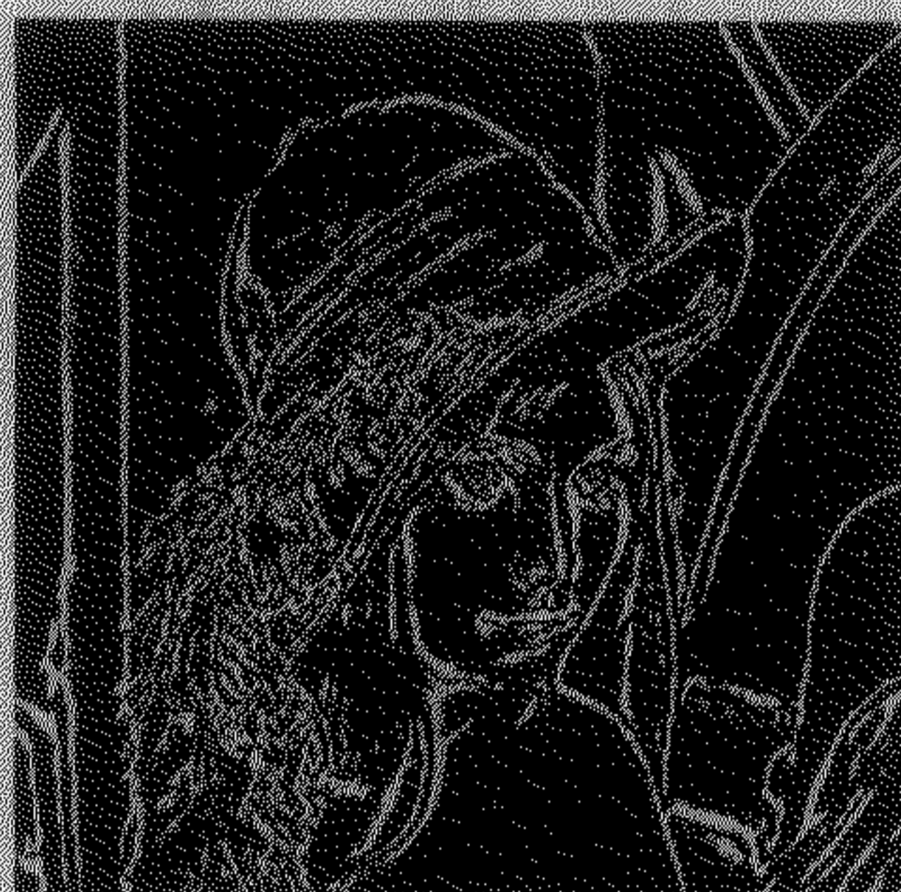
Figure 3.3: Edge detection neural learning when target was edge image by LoG operator.
