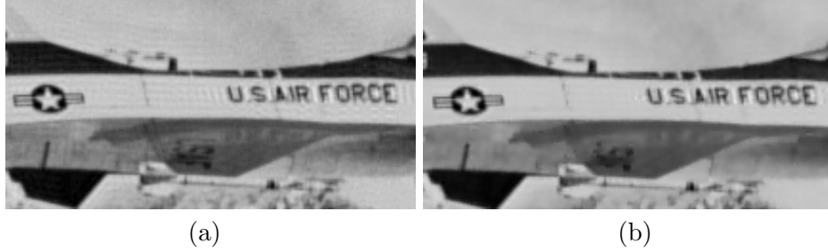
Figure 2.3: (a) Scaled and cropped SR output of iterative algorithm. (b) After smoothing by some adaptive spatial domain filtering technique
