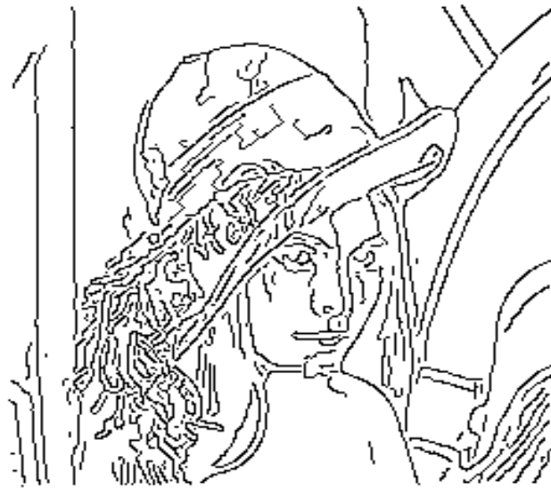
Fig. 6 (c) Result of applying Sarif et al.'s method with h = 1.25 , Tl = 5 , Tu = 30 on the LENA image (color)
