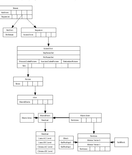
Figure 3.2: H.264/AVC coded data structure
