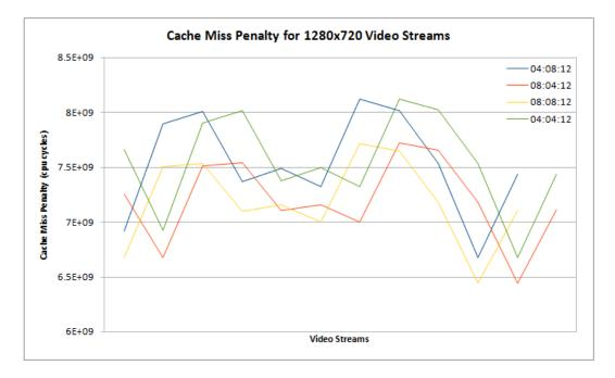
Figure 5.2: Graph representing Cachemisspenalty to decode coded video streams of resolution 1280x720(04:04:12 represents associativity of 11 cache is 4; D1 cache is 4 and for L3 cache associativity is 12)
