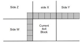
Figure 4.1: A 4x4 Block with neighbouring 13 samples
