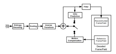
Figure 3.1: Block Diagram of H.264 Decoder
