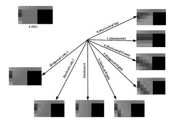
Figure 4.2: Direction of dependency for different prediction modes of Intra 4x4 Prediction for luma samples
