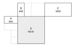
Figure 3.7: Neighbouring partitions for motion vector prediction when partition sizes are different
