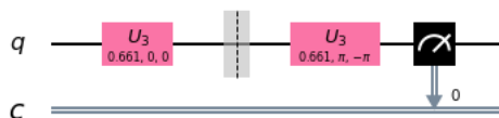
Figure 4-3: Circuit diagram of the QSDC protocol executed on the IBMQ Armonk device
