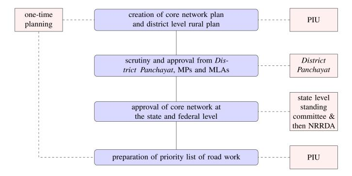
Figure 4.1: Preliminary Stages of PMGSY Road Planning (One Time Design)
