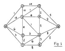
Let the points (cities) at which the maintenance is available be denoted by 2, 4, 6, 8. Our object is to trace the path from 0 to any of these cities so as to maximise the total profit given by the vehicle. The values of d (i, j) are given in Fig. I.
