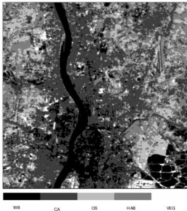
Fig. 5. Segmented output of Calcutta IRS-1A image using average and busyness as features with c = 5 ( \beta = 2.84578 )
