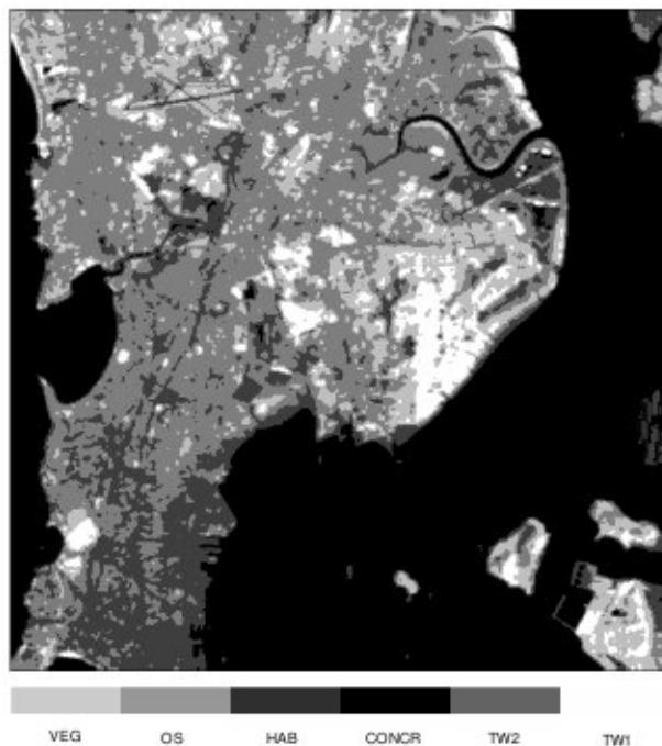
Fig. 9. Segmented output with c = 6 with average and busyness as features ( \beta = 7.21309 )
