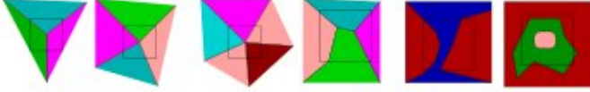
Fig. 1. Examples of three types of junctions where multiple region merges and three examples of presence of parts of different image segments in an image neighborhood. A rectangular window in each case shows the region of interest.
