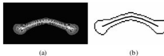
Fig. 3: (a) The (0-1) normalized curvature map \hat{\Psi} of the regularized gradient vector field \vec{G} of Fig. 2. Lighter shades indicate values closer to 1; (b) Centerline of the \mu -level set of \hat{\Psi} ( \mu=0.1 ) of (a).
