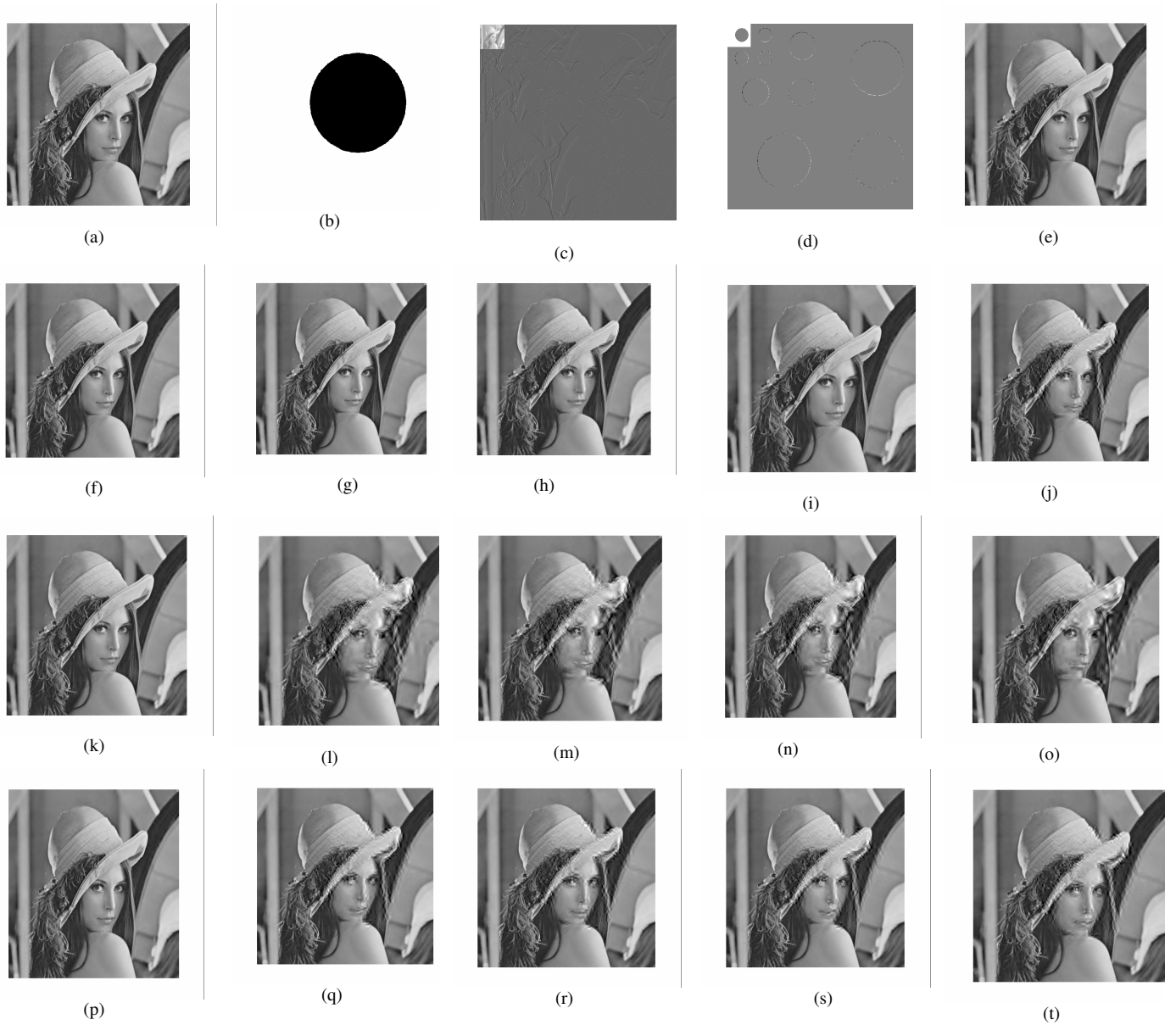
Fig. 7: (a) original image, (b) binary mask, (c) 3-scale lifting transformation of original image (a), (d) 3-scale lifting transformation of binary mask (b), (e) decoded image without quality control scheme, (f) & (g): quality accesses control for case-1, (f) decoded image without key, (g) decoded image with the true key, (h) & (i): accesses control for case-2, (h) decoded image without key, (i) decoded image with the true key, (j) & (k): accesses control for case-3, (j) decoded image without key, (k) decoded image with the true key, (l)– (p): results when original image goes through 4-scale lifting transformation and all detail subbands are modulated, (l) decoded image without key (PSNR=23.8568, SSI=0.7381), (m) output when detail coefficients of level-1 are decoded with true key (PSNR=24.0257, SSI=0.7598), (n) output when detail coefficients of level-1 and 2 is decoded with true key (PSNR=24.5767, SSI=0.7951), (o) output when detail coefficients of level-1, 2 and 3 are decoded with true key (PSNR=26.6225, SSI=0.8504), (p) output when detail coefficients of level-1, 2, 3 and 4 are decoded with true key (PSNR=34.0996, SSI=0.9079). (q)–(t): Results if “Lena” image is decoded by different false (a random) key (for case-3), (q): decoded image with false key (1 st try) (PSNR=26.7177 dB, SSI=0.7910), (r): decoded image with false key (2 nd try) (PSNR=26.7145 dB, SSI=0.7898), (s): decoded image with false key (3 rd try) (PSNR=26.6689 dB, SSI=0.7905), (t): decoded image with false key (4 th try) (PSNR=26.7415 dB, SSI=0.7918).
