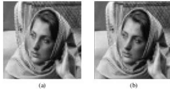
Fig. 8. (a) Image reconstructed from only the approximation component in the case of PRF4 set of ISITRA (last entry in Table 3). (b) Image reconstructed from only the approximation component in the case of DB2 wavelet filters.
