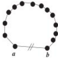
Fig. 3. An example showing that although the distance ab is greater than thresh , the cluster will not be split.
