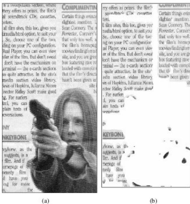
Fig. 10. (a) Test image with nonconvex and overlapping object boundaries. (b) Segmented result.
