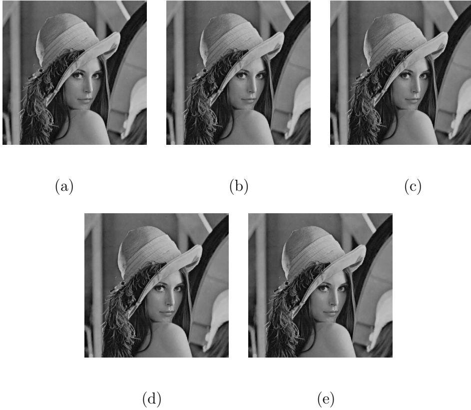
Figure 3.5: The step-by-step effect of 2BTC-PFG on ‘Lena’: (a) BTC (PSNR=32.89 dB, bpp=2.00), (b) PF- A-d (PSNR= 31.79 dB, bpp= 1.375) (c) PF- A-d' (PSNR= 31.61 dB, bpp= 0.88) (d) CONM (PSNR= 31.57 dB, bpp= 0.64) (e) INTM (PSNR= 31.59 dB, bpp= 0.64).
