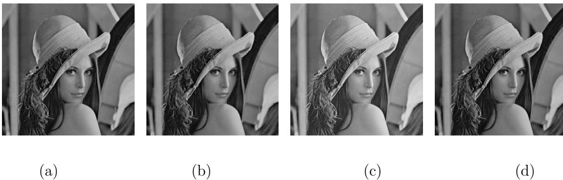
Figure 3.9: Step-by-step results of LBTC-PF method on ‘Lena’: (a) BTC (PSNR = 32.89 dB, bpp = 2), (b) QS-BTC (PSNR = 30.36 dB, bpp = 1), (c) QS-PF (PSNR = 29.56 dB, bpp = 0.53), (d) QS-PF- d' -IG (PSNR = 29.43 dB, bpp = 0.39).
