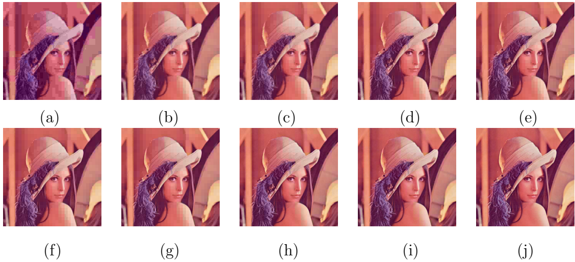
Figure 5.10: Reconstructed images by CPBTC-PF method at different stages: (a) Stage 1: PSNR=22.597 dB, Cbpp=0.159, (b) Stage 2: PSNR=25.774 dB, Cbpp=0.301, (c) Stage 3: PSNR=26.208 dB, Cbpp=0.446, (d) Stage 4: PSNR=27.122 dB, Cbpp=0.518, (e) Stage 5: PSNR=27.745 dB, Cbpp=0.566, (f) Stage 6: PSNR=28.592 dB, Cbpp=0.614, (g) Stage 7: PSNR=28.978 dB, Cbpp=0.676, (h) Stage 8: PSNR=30.302 dB, Cbpp=1.029, (i) Stage 9: PSNR=31.128 dB, Cbpp=1.339, (j) Stage 10: PSNR=32.185 dB, Cbpp=1.593.
