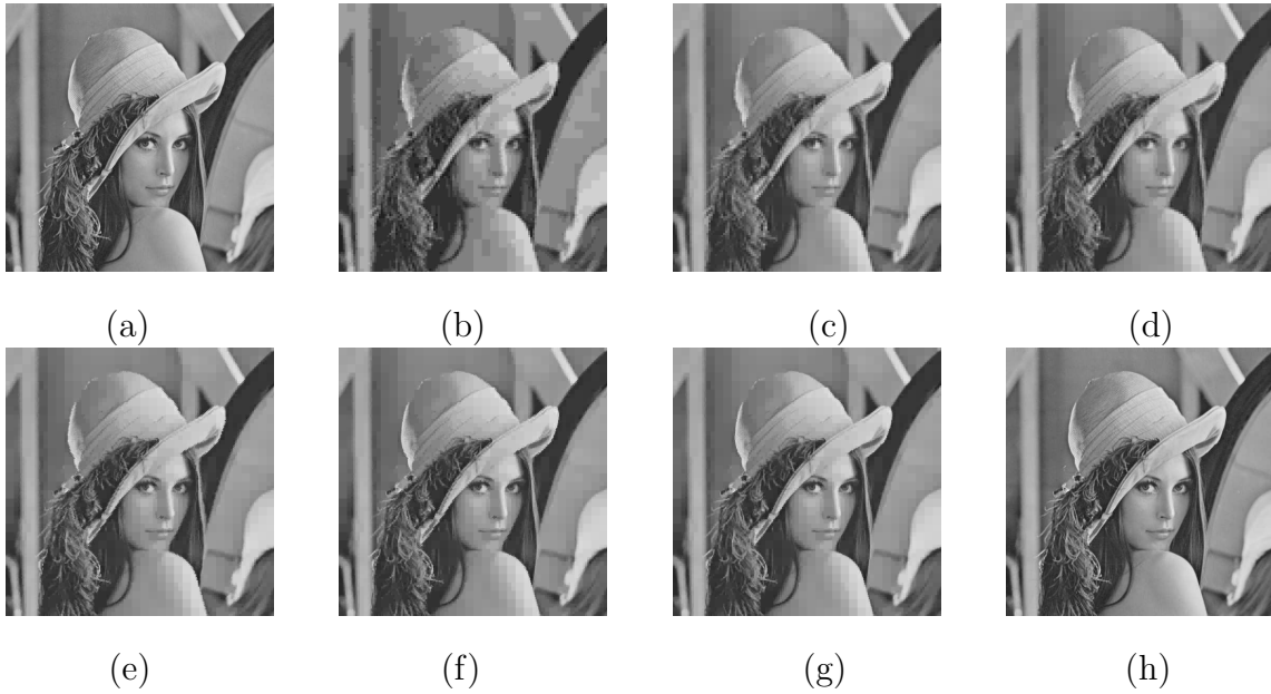
Figure 5.7: (a) Original Image, (b)-(g) Reconstructed images in Phase I: (b) Stage 1: PSNR= 24.817 dB, Cbpp = 0.133, (c) Stage 2: PSNR= 26.629 dB, Cbpp = 0.252, (d) Stage 3: PSNR= 27.227 dB, Cbpp = 0.404, (e) Stage 4: PSNR= 28.687 dB, Cbpp = 0.480, (f) Stage 5: PSNR= 29.715 dB, Cbpp = 0.530, (g) Stage 6: PSNR= 31.279 dB, Cbpp = 0.580, (h) Reconstructed images in Phase II: PSNR= \infty , Cbpp = 4.432.
