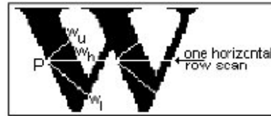
Fig. 5. Detection of bold characters: thickness at a stroke boundary point
