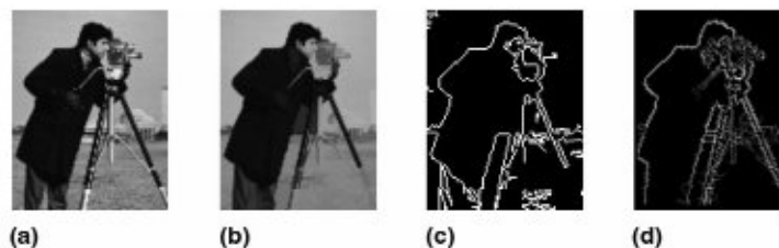
Fig. 4. (a) Cameraman image, (b) after AOC operation on (a) at a = 100 , (c) edge image from (b) using (6) (edges shown in white), (d) edge map using (Canny, 1986) at \sigma = 1 .
