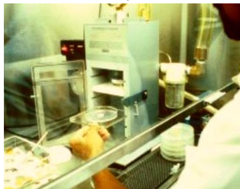
An IRRI biotechnology laboratory where foreign genes are introduced into rice cells using biolistic process. Courtesy of CGIAR Photo Library
