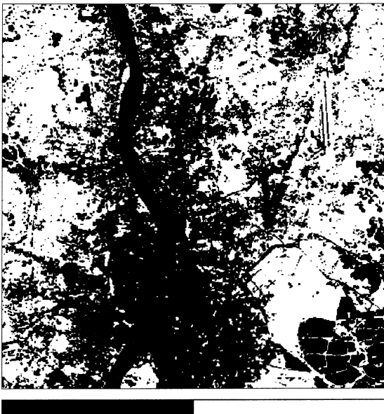
Fig. 3. Segmentation of the Calcutta image using HCM with c = 2 .
