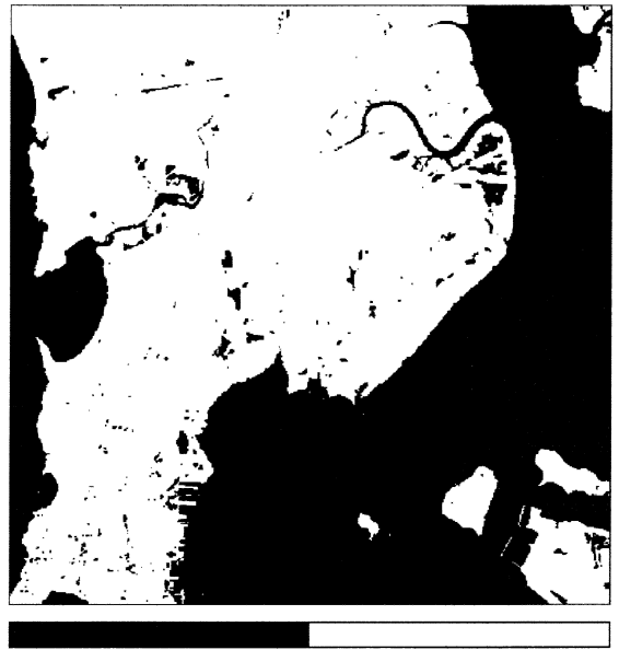
Fig. 4. Segmentation of the Bombay image using HCM with c = 2 .
