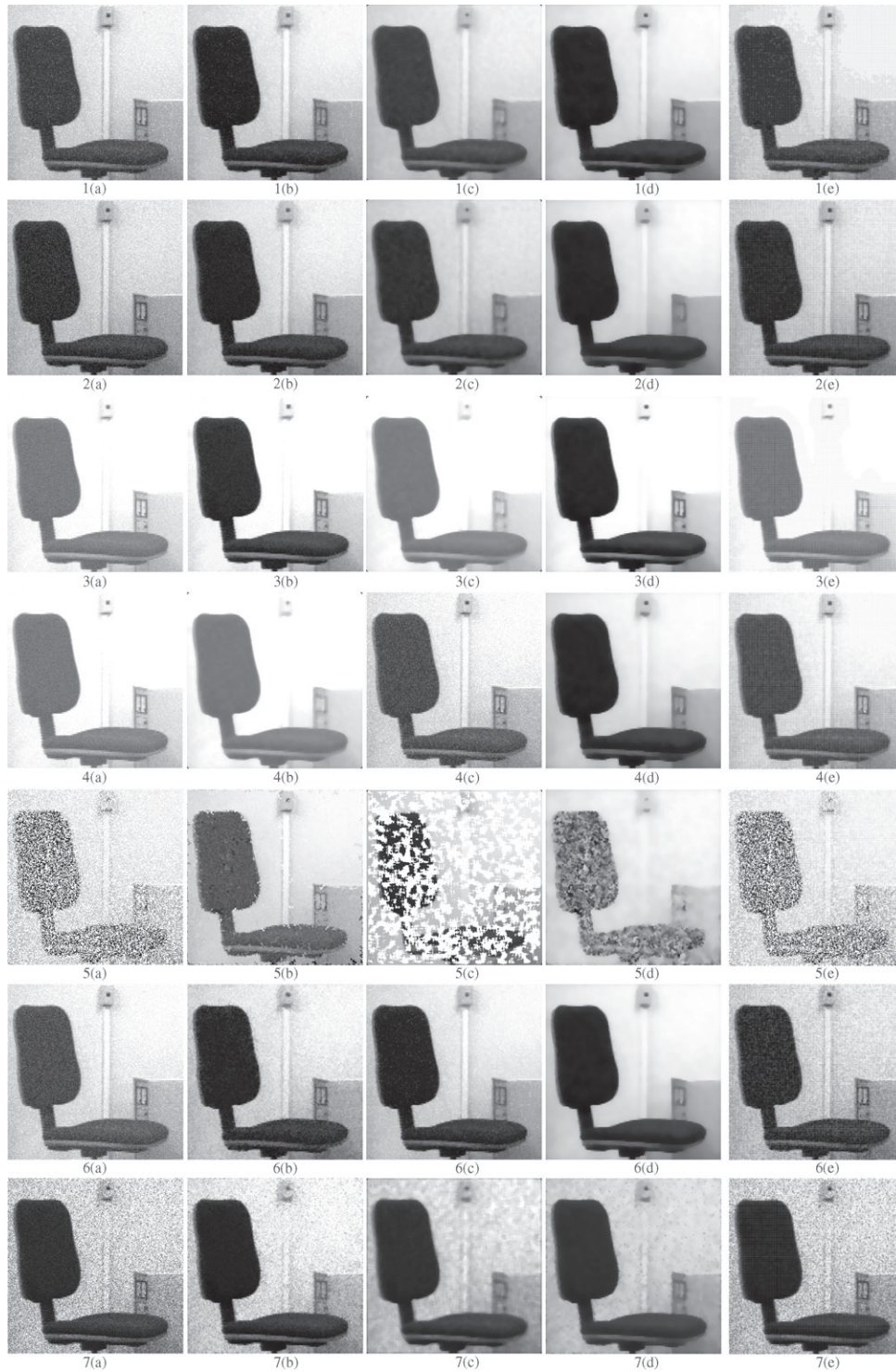
Fig. 5. (a) Original noisy image; (b) result of proposed multiscale morphological noise removal filtering; (c) result of median filtering; (d) result of Crimmins algorithm; (e) results of anisotropic diffusion smoothing. (1) Exponential noise; (2) Gaussian noise; (3) Poisson noise; (4) Rayleigh noise; (5) shot noise; (6) uniform noise; (7) speckle noise.
