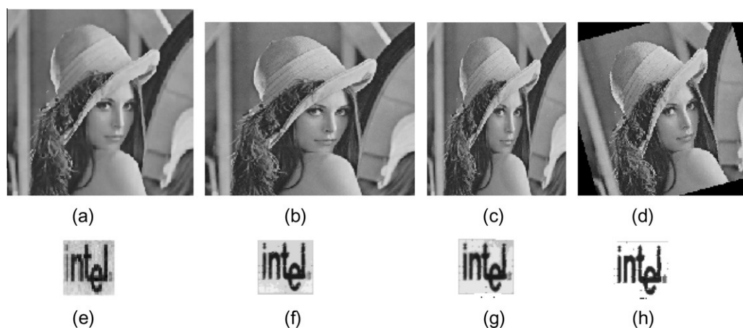
Fig. 7. (a) Watermarked image after wiener filtering with window size (5 \times 5) , (b) watermarked image after change in aspect ratio ( X = 1.0, Y = 1.2 ), (c) watermarked image after change in aspect ratio ( X = 1.2, Y = 1.0 ), (d) watermarked image after 15^\circ rotation (e) extracted watermark from (a), (f) extracted watermark from (b), (g) extracted watermark from (c), (h) extracted watermark from (d).
