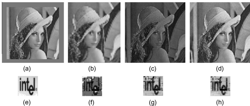
Fig. 6. (a) Watermarked image after symmetric cropping operation, (b) watermarked image after rescaling from its one-fourth size, (c) watermarked image after sharpening operation, (d) watermarked image after noise addition, (e) extracted watermark from (a), (f) extracted watermark from (b), (g) extracted watermark from (c), (h) extracted watermark from (d).
