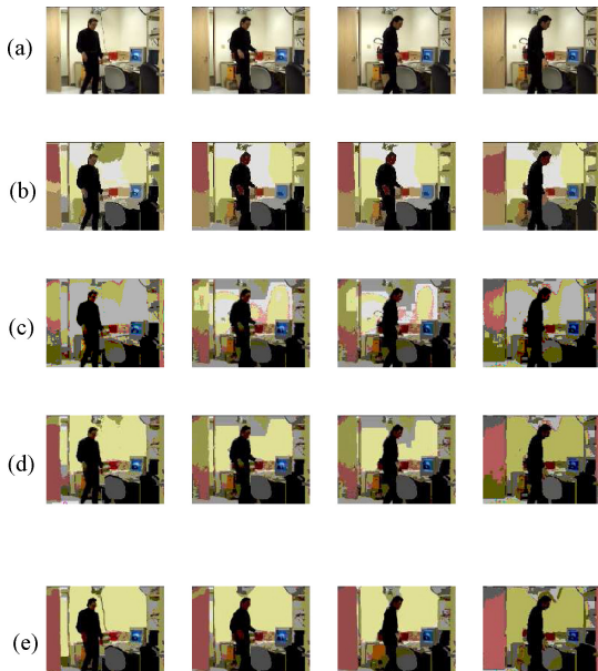
Fig. 4. Spatial segmentation of frame numbers 1857th, 1858th, 1859th, and 1860th of the LightSwitch video sequence. (a) Original frames. (b) Spatial segmentations using meanshift scheme. (c) Spatial segmentations using only MRF model. (d) Spatial segmentations using MRF and deterministic kernel-based local edge prior. (e) Spatial segmentations using proposed fuzzy kernel-based local edge prior.
