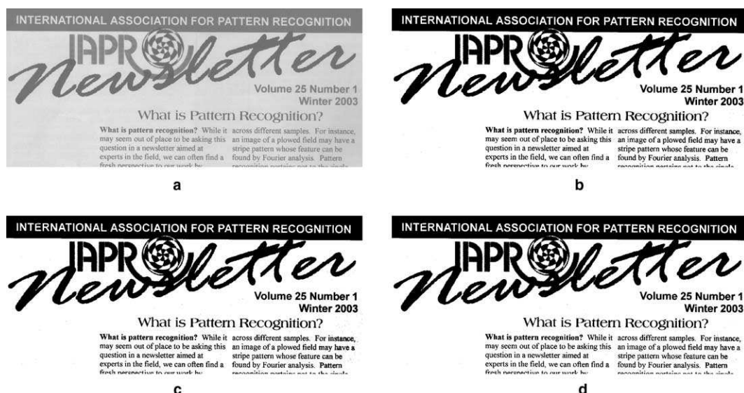
Fig. 7. Thresholds by maximizing rough entropy using granule of different sizes on TEXT image: (a) original, (b) threshold = 169, granule size = 15 \times 15 , (c) threshold = 171, granule size = 10 \times 10 , (d) threshold = 168, granule size = 19 \times 19 .
