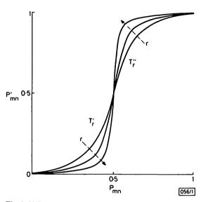
Fig. 1 INT transformation function for contrast enhancement
