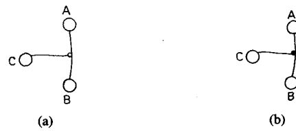
Fig. 16. (a) A stimulating modifier of the link connecting the nodes A and B, (b) A deactivating or inhibitory modifier of the link connecting the nodes A and B.
