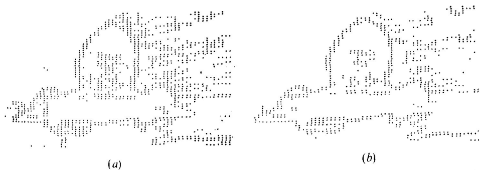
Figure 10. (a) Thresholded version of Fig. 8(c) using normal histogram thresholding techniques when thresholded at edge intensity level 4; (b) thresholded version of Fig. 8(c) using the same technique with level of threshold 6.
