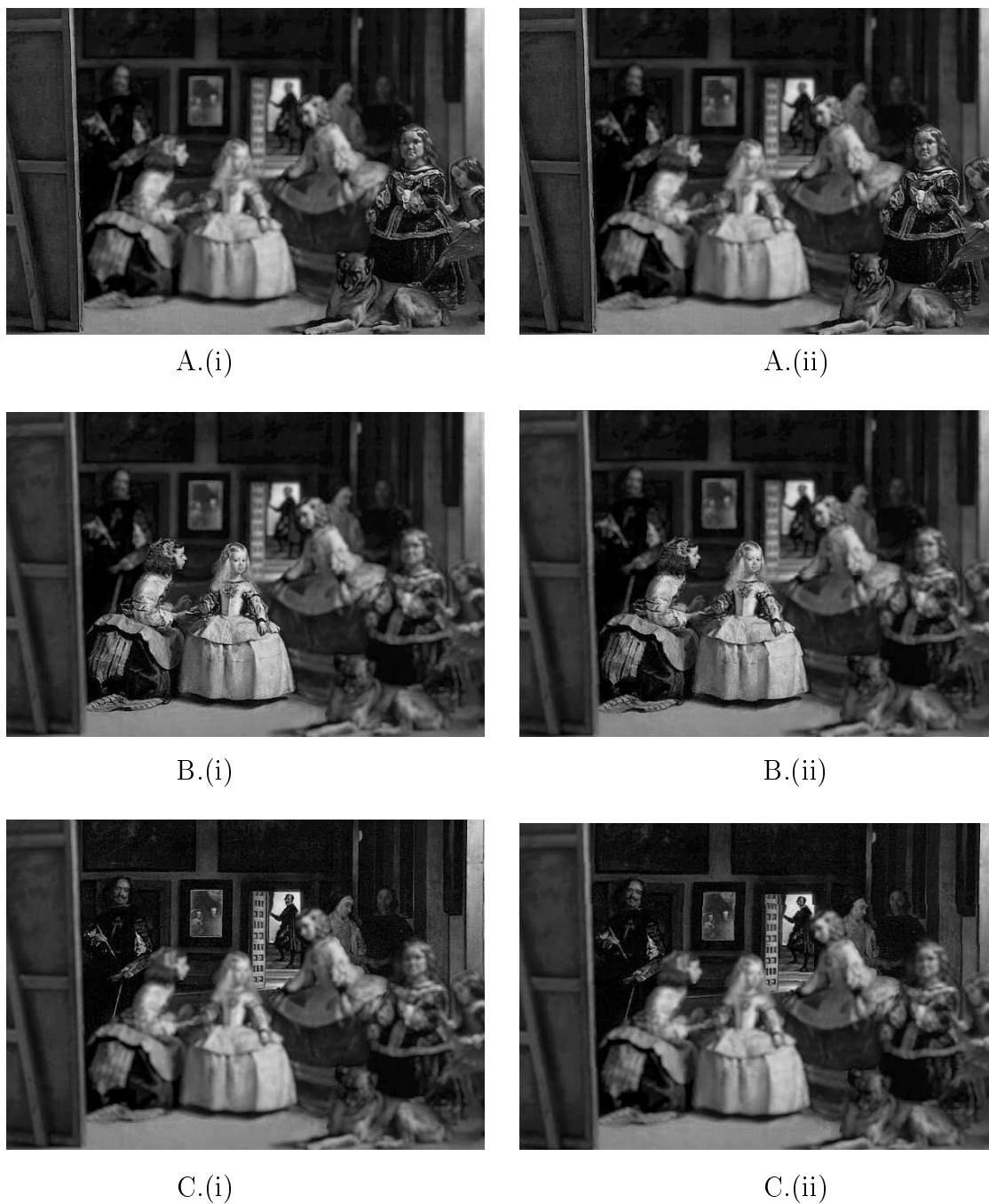
Figure 2.4: 'Doll': Original, Registered and Difference images. A.(i) Near-focused image (reference-image), A.(ii) Truncated near-focused image (new reference-image), B.(i) Middle-focused image, B.(ii) Registered middle-focused image, C.(i) Far-focused image, C.(ii) Registered far-focused image, D. Difference between A.(i) & B.(i), E. Difference between A.(i) & C.(i), F. Difference between A.(ii) & B.(ii), G. Difference between A.(ii) & C.(ii)
