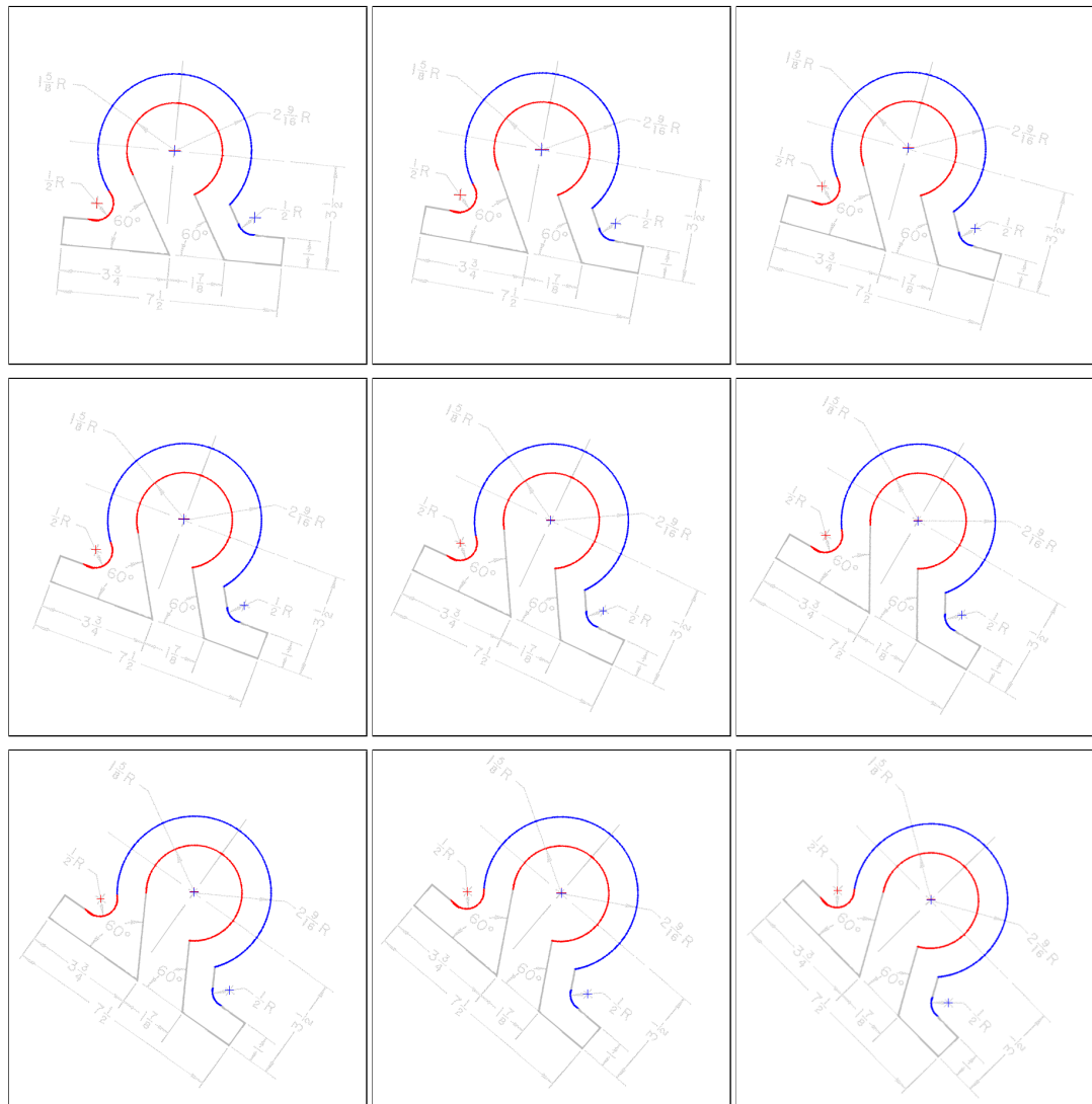
Figure 2.12: Results showing robustness of our algorithm against rotation. The output images are for g07-tr6.tif , rotated clockwise by 5^\circ , 10^\circ , 15^\circ , ..., 45^\circ , shown here in row-major order.
