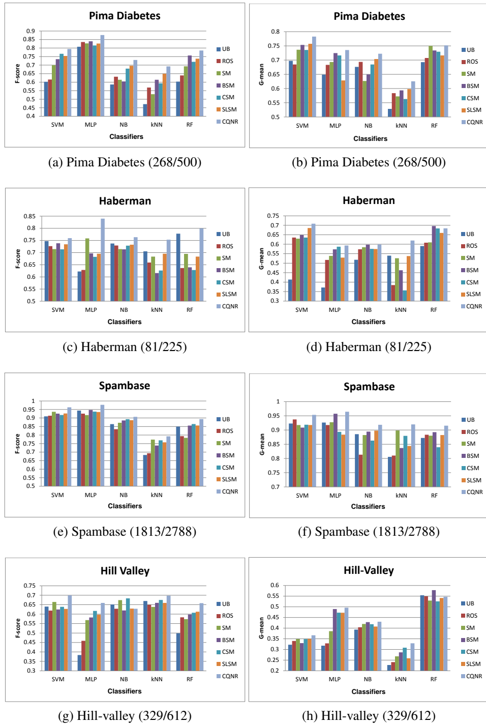
Figure 4.4: Comparison of the classification performances, in terms of F -score and G -mean, of different classifiers on datasets oversampled by different oversampling algorithms. The numbers within brackets indicate the ratio of the cardinalities of minority class to the majority class. The abbreviations for the methods are UB - imbalanced, ROS - Random Oversampling, SM - SMOTE, BSM - borderline SMOTE, CSM - C Smote, SLSM - Safe level SMOTE, CQNR - Cluster Quality-based Non-Reductional Oversampling. As observed from the figures, CQNR has performed the best over the other oversampling algorithms considered here.
