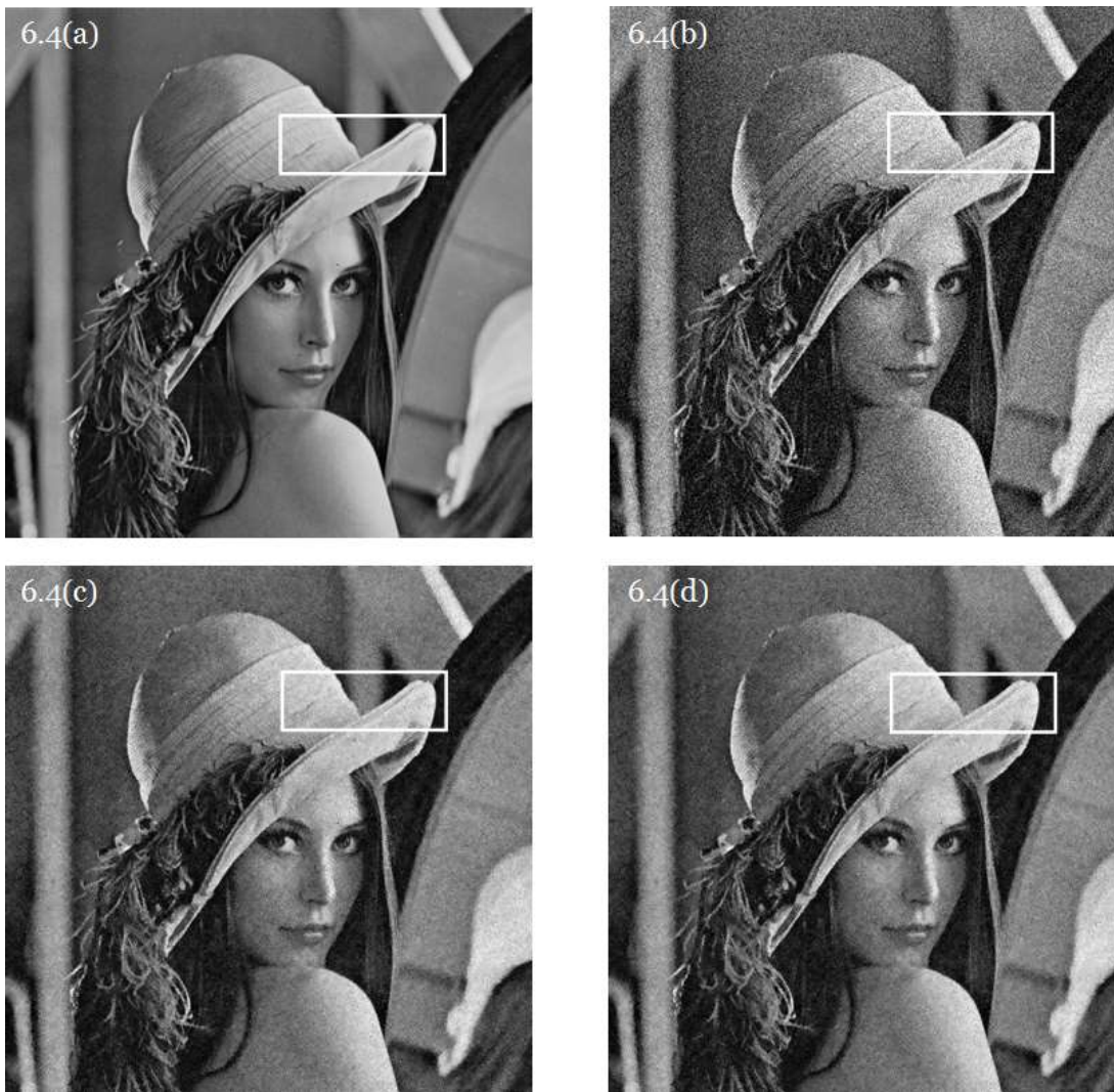
Figure 6.4 (a) Lena.jpg 512 x 512 grayscale image. (b) Lena image with additive white Gaussian noise of variance 0.01. (c) M-channel filter result on Figure 6.4(b). (d) Bilateral filter (spatial-domain standard deviation = 3 and the intensity-domain standard deviation = 0.1) result on Figure 6.4(b). The region of interest has been marked using a white rectangle in each figure.
