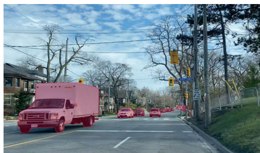
(b) Example of instance segmentation: Uniquely identifying vehicles which are cars, motorcycles, buses, and so on. Each vehicle is treated uniquely.
